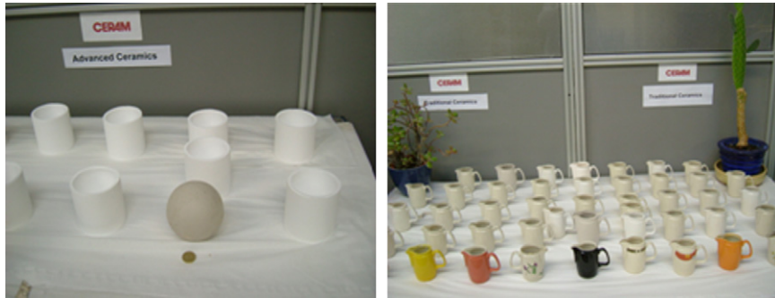
Fig. 3. Hollow ceramic items produced by the ICRM route.
